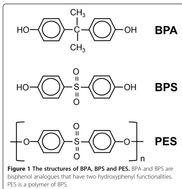
**Figure 1** The structures of BPA, BPS and PES. BPA and BPS are bisphenol analogues that have two hydroxyphenyl functionalities. PES is a polymer of BPS.
